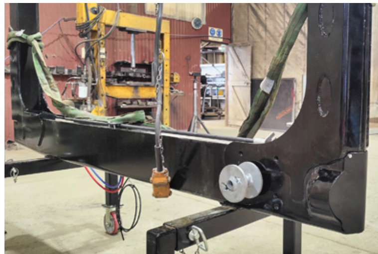
^ Building the tensioner into the bolster base at Trinder Engineers.
