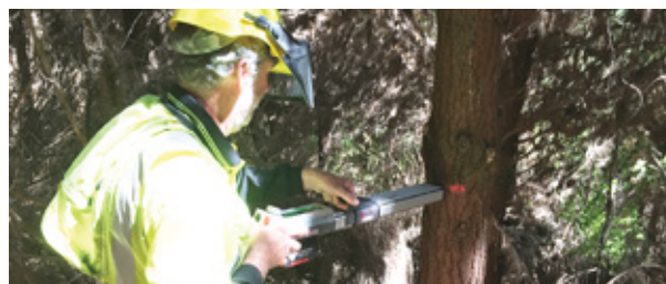
^ Paul Thompson of Buck Forestry using an IML Resistograph to test basic corewood density
