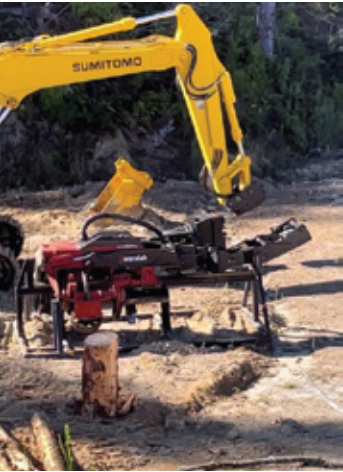
^ Picking up a processing head with the quick coupler.
