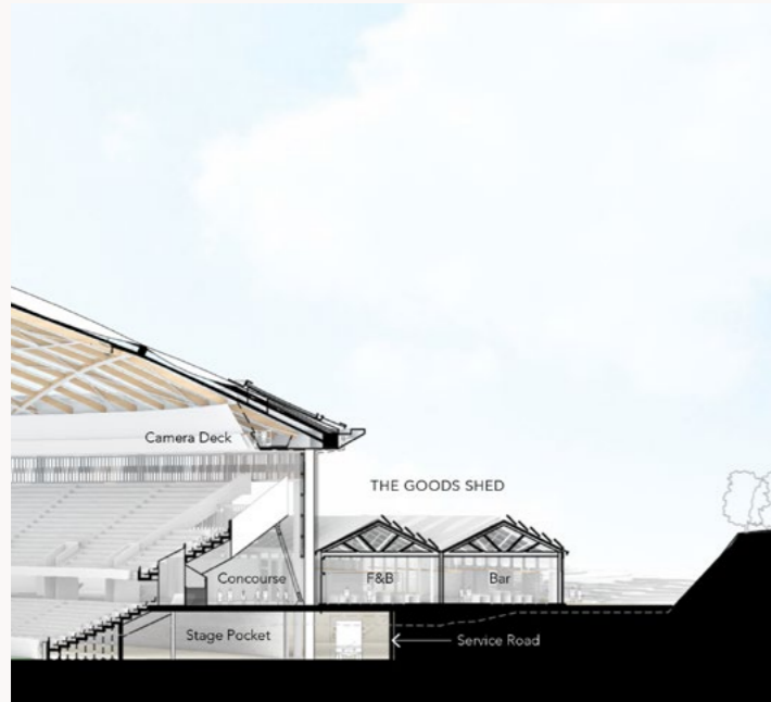
Section through Northern Stand and Good Shed
